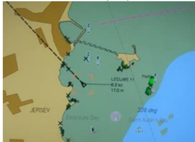
FIG 24 & 25 L'ECUME II having passed south of the outlying rocks crosses the 0m sounding and then runs aground at 8 knots.
