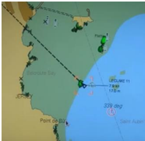
FIG 24 & 25 L'ECUME II having passed south of the outlying rocks crosses the 0m sounding and then runs aground at 8 knots.
